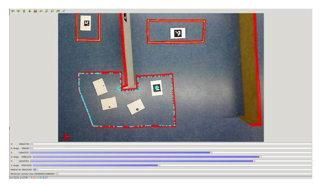
the currently selected contour is now highlighted in torques. It can now be saved by pressing *s* on the keyboard. The Terminal in which the *calibrate\_scene.py* script was called will now ask for a file name. If provided it saves the contour as a *.npy* object.
