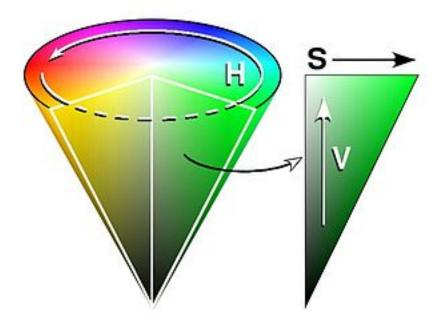
For OpenCV, The Hue Range goes from 0-179 (which is half that of the common Hue definition which goes from 0 to 359). since the Hue value is cyclical, both these values represent a type of red. While the borders between colors are not clearly defined the following table gives an idea which hue values to pick for each object color
