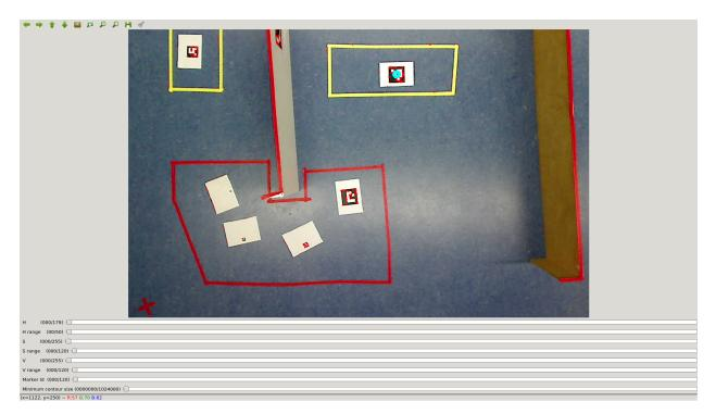
The first six sliders are used to select the color of the desired object. This color is specified in the HSV colorspace. HSV refers to Hue, Saturation, and Value. A good visualization of the HSV values can be seen in this image from its wikipedia page:
